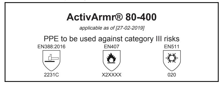
is in conformity with the provisions of Regulation (EU) 2016/425 and with the European harmonised standards EN420:2003+A1:2009, EN388:2016, EN407, EN511, and is identical to the PPE which is subject to the EU Type Examination (Module B, Annex V of the Regulation); under certificate number 032/2019/0340 issued by the Notified Body:
