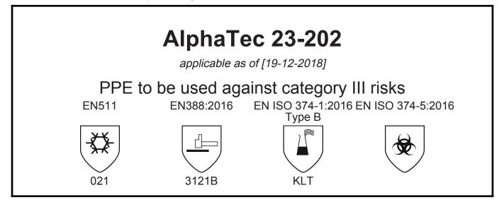
is in conformity with the provisions of Regulation (EU) 2016/425 and with the European harmonised standards EN420:2003+A1:2009, EN511, EN388:2016, EN ISO 374:2016, and is identical to the PPE which is subject to the EU Type Examination (Module B, Annex V of the Regulation); under certificate number 032/2018/2165 issued by the Notified Body:
